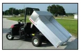
Tilt for dumping and engine access
