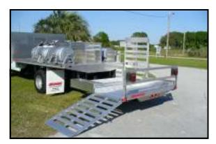
Spray truck dual rear spreader platform with side load ramps and bucket rack
