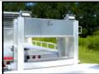
Upper GN Box & loading lights
